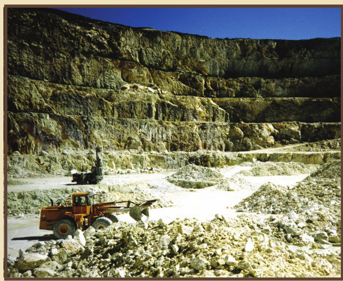
View of Canada's only producing pyrophyllite mine, showing the benches cut in the quarry face.
